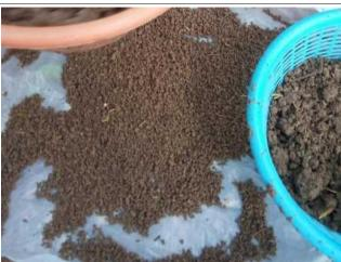
2) take local clay soil, sift the soil to get around 2 kg of small particle clay soil
