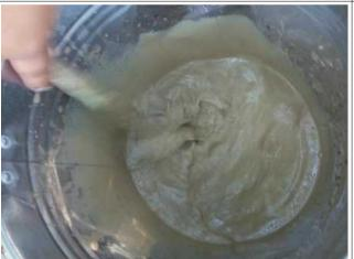
3) mix well the potassium permanganate solution with the clay soil
